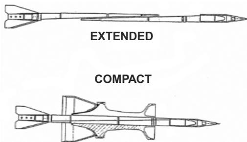
The concept can yield significant increases in penetration depth while still fitting into an appropriate delivery vehicle. The penetrator is launched in the “Compact” form, and converts to the “Extended” form shortly before impact.
