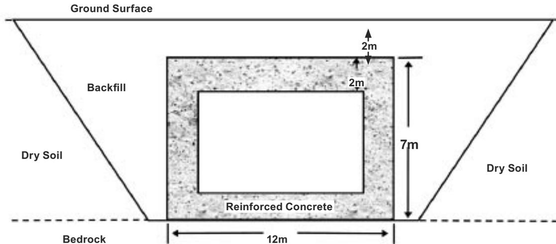
An area is dug out of the surrounding soil, the reinforced concrete bunker is built in the open pit, and the dug-out area is filled in.
